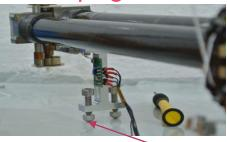
Test performed on the epoxy floor, using Miniature Ball Transfer Units (BTU)- Og facility
